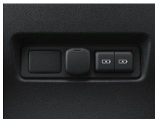
Accessory socket (DC12V/120W) H - Rear of center console box
