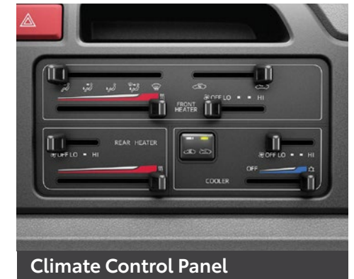
Climate Control Panel Redesigned for ease of use The climate control panel provides excellent visibility and ease of use.
